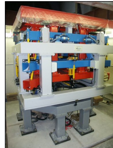
6 component underfloor balance –Aerotech ATE, Ltd.
